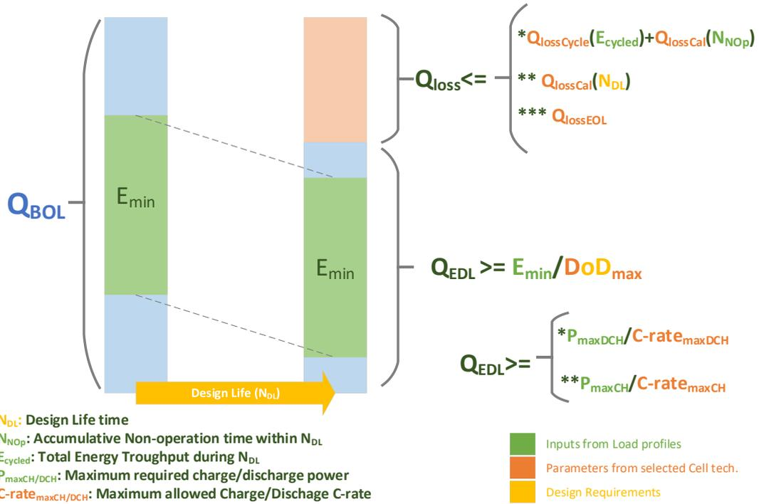
FIG. 6.7: ILLUSTRATION OF ESS SIZING CRITERIA
