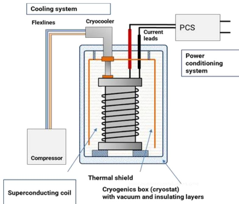
**FIG. 4.1: GENERAL SMES STRUCTURE WITH A DRY COOLING SYSTEM**
