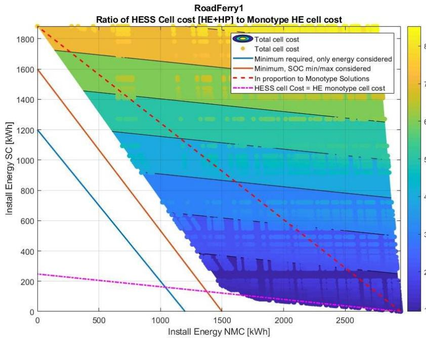
**FIG. 10.16: HESS SCREENING RESULTS FOR RO-RO FERRY 1 CASE WITH NMC BATTERIES AND SC. (SC & NMC DESIGN LIFE = 7.5 YEARS)**
