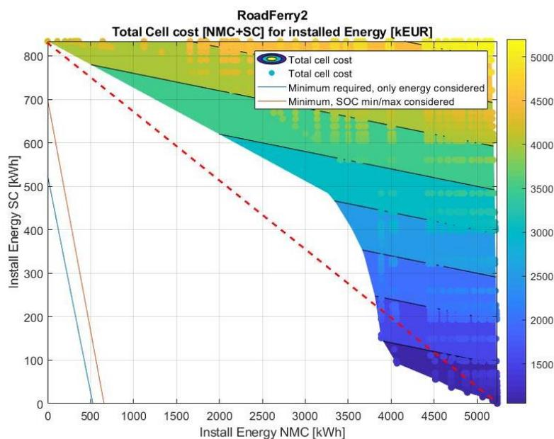
**FIG. 10.19: HESS SCREENING RESULTS FOR RO-RO FERRY 2 CASE WITH NMC BATTERIES AND SC. (SC & NMC DESIGN LIFE = 7.5 YEARS)**
