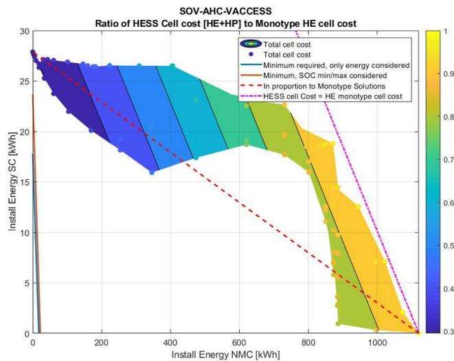
**FIG. 10.43: HESS SCREENING RESULTS FOR OSV-AHC CASE WITH NMC BATTERIES AND SC. GENSET LFP = 0,01Hz. (SC & NMC DESIGN LIFE = 7.5 YEARS)**
