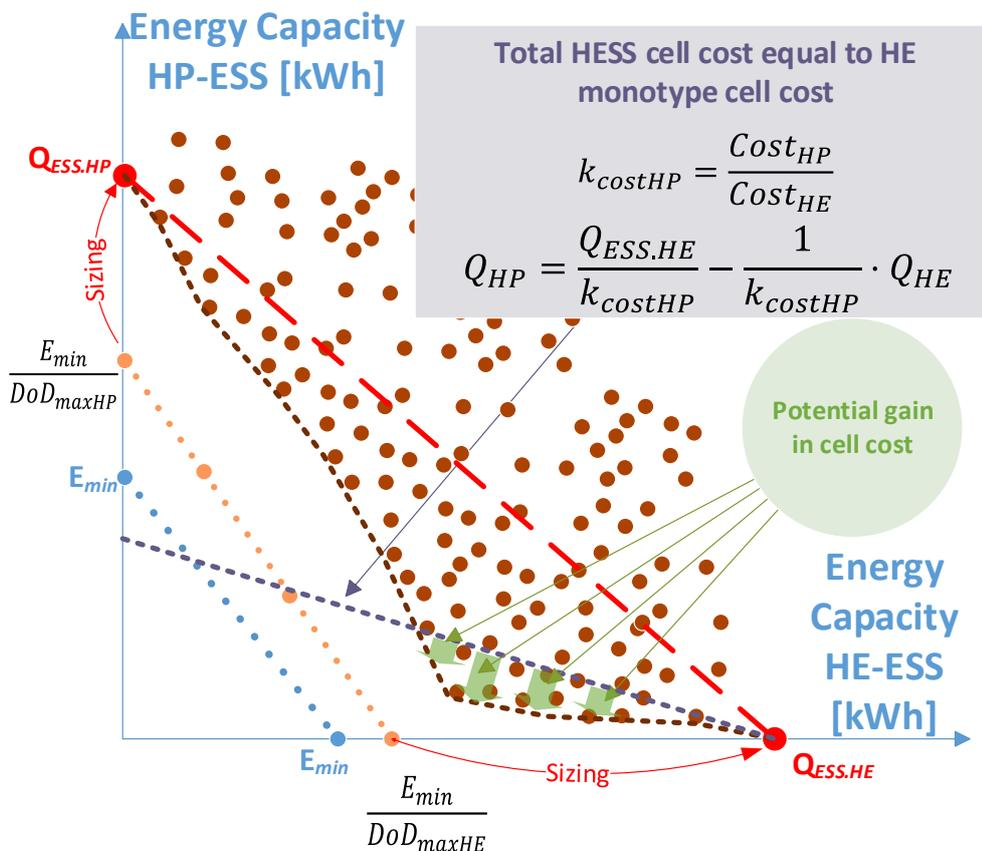
FIG. 6.10: EXAMPLE OF A HESS POWER PROFILE WITH SOME HESS SOLUTIONS SHOWING POTENTIAL REDUCTION IN CAPITAL COST.
