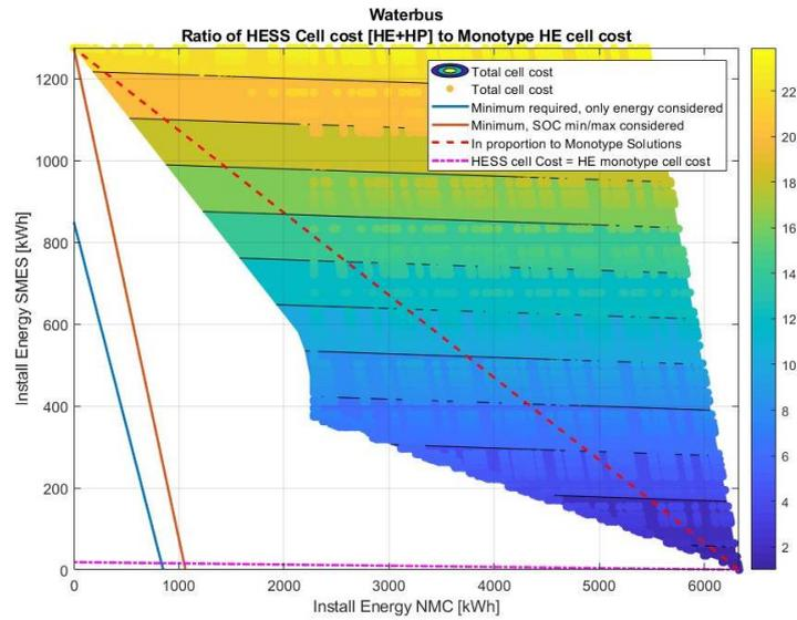
**FIG. 10.28: HESS SCREENING RESULTS FOR WATER BUS CASE WITH NMC BATTERIES AND SMES. (NMC DESIGN LIFE = 10 YEARS)**
