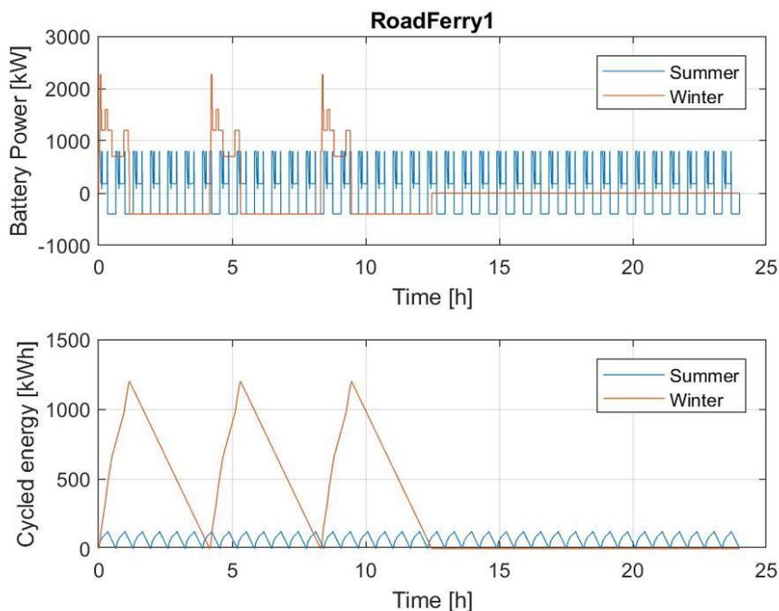
charger is available at each ferry station, so the HESS recharge the energy consumed after each trip section. The cycled energy, estimated from the power time series is also shown in Fig. 6.3.
