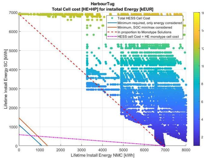
**FIG. 10.22: HESS SCREENING RESULTS FOR HARBOUR TUG CASE WITH NMC BATTERIES AND SC. LIFETIME INSTALLED CAPACITY FOR DIFFERENT DESIGN LIFE: NMC → 5-15 YEARS AND SC → 5- 7.5 YEARS.**
