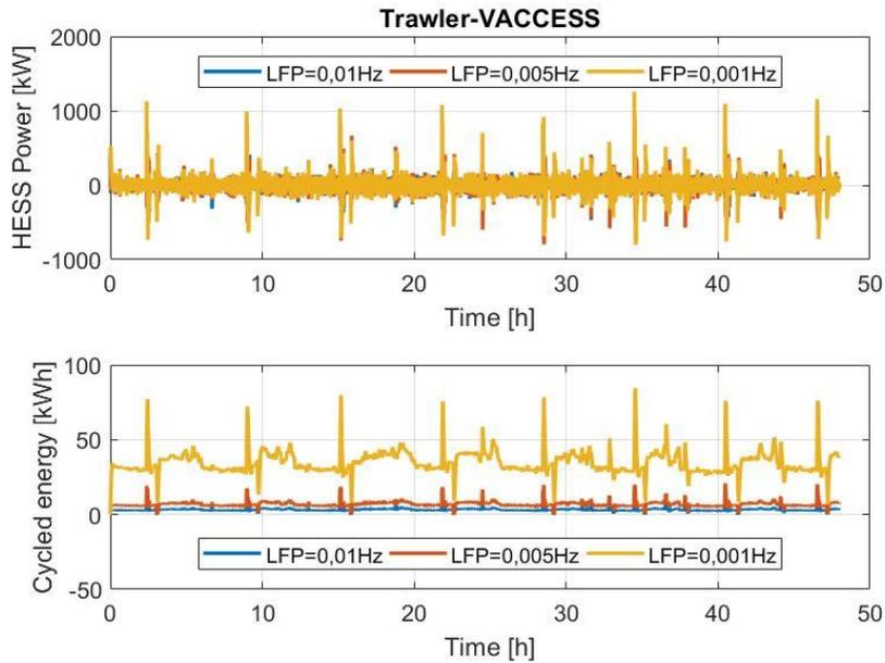
**FIG. 10.13: POSSIBLE TRAWLER HESS POWER PROFILE FOR DIFFERENT LOW PASS FILTERS**
