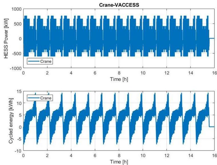
**FIG. 10.39 BULK CARRIER WITH CRANE OPERATION - TYPICAL PROFILE**
