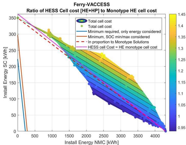
**FIGURE 10.6: HESS SCREENING RESULTS FOR FERRY CASE WITH NMC BATTERIES AND SUPERCAPACITORS. RESULTS FOR NMC DESIGN LIFE OF 10 YEARS AND SC DESIGN LIFE OF 7.5 YEARS.**
