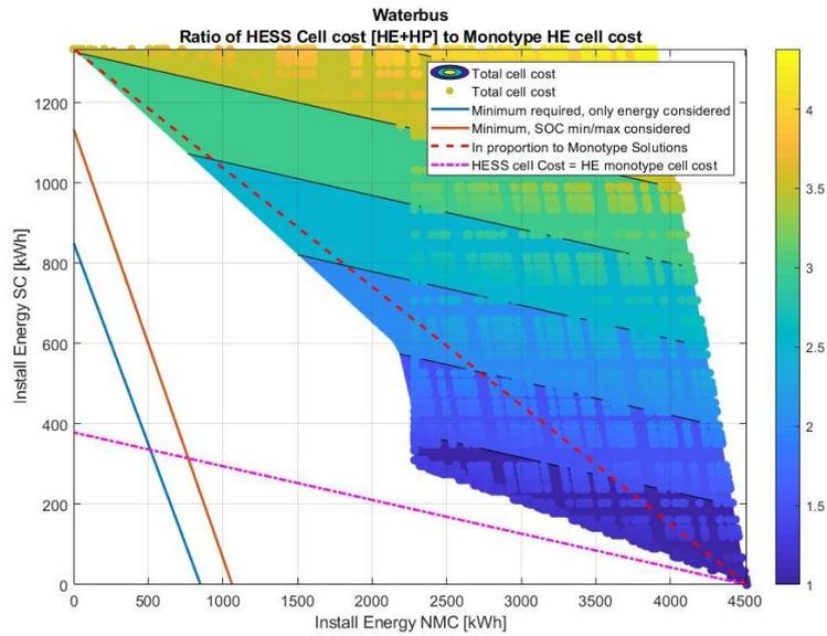
**FIG. 10.26: HESS SCREENING RESULTS FOR WATER BUS CASE WITH NMC BATTERIES AND SC. (SC & NMC DESIGN LIFE = 7.5 YEARS)**
