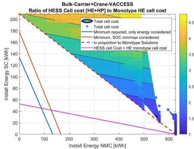
**FIG. 10.40: HESS SCREENING RESULTS FOR BULK CARRIER CRANE OPERATION CASE WITH NMC BATTERIES AND SC. (SC & NMC DESIGN LIFE = 7.5 YEARS)**
