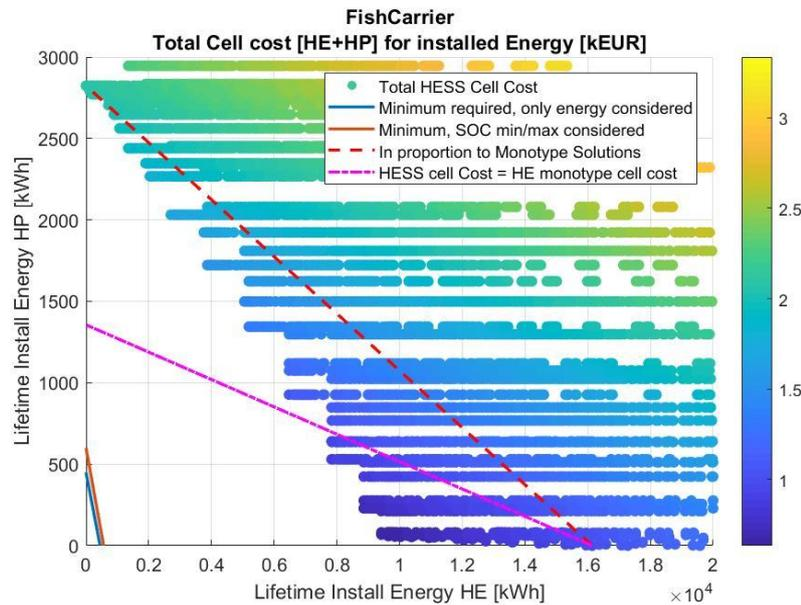
**FIG. 10.33: HESS SCREENING RESULTS FOR FISH CARRIER CASE WITH NMC BATTERIES AND SC. LIFETIME INSTALLED CAPACITY FOR DIFFERENT DESIGN LIFE: NMC → 5-15 YEARS AND SC → 5- 7.5 YEARS.**
