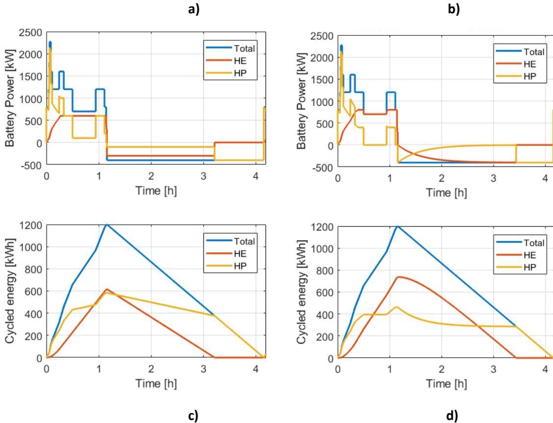
**FIG. 6.5: EXAMPLE OF TIME SERIES OBTAINED BY THE POWER SPLIT ALGORITHM WITH A)  $F_0=50\text{MHz}$ ,  $P_{HE.DCHmx} = 600\text{kW}$ ,  $P_{HE.CHmx} = 300\text{kW}$ ; B)  $F_0= 100\text{MHz}$ ,  $P_{HE.DCHmx} = 600\text{kW}$ ,  $P_{HE.CHmx} = 300\text{kW}$ ; C)  $F_0= 100\text{MHz}$ ,  $P_{HE.DCHmx} = 600\text{kW}$ ,  $P_{HE.CHmx} = 300\text{kW}$ ; AND D)  $F_0= 100\text{MHz}$ ,  $P_{HE.DCHmx} = 800\text{kW}$ ,  $P_{HE.CHmx} = 400\text{kW}$ ;**
