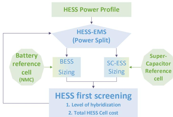
**FIGURE 6.2: SIMPLIFIED HESS EVALUATION FRAMEWORK FOR FIRST SCREENING. NMC VS SC TECHNOLOGIES.**
