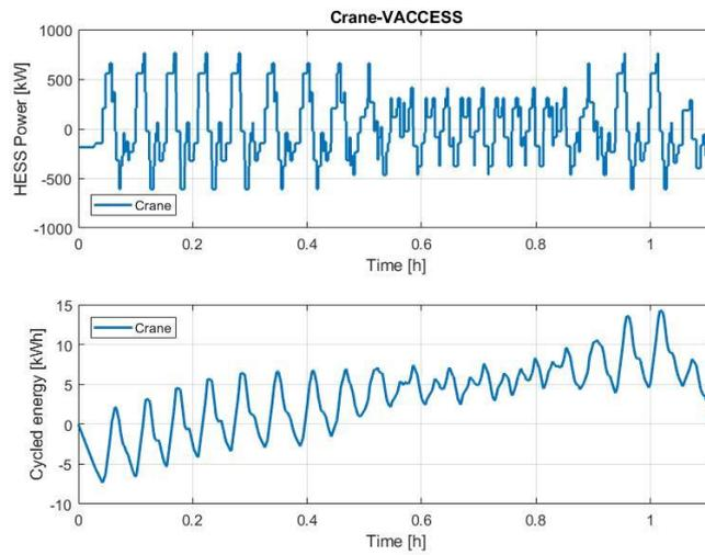
**FIG. 10.38: BULK CARRIER WITH CRANE OPERATION - HESS FUNDAMENTAL CYCLE**
