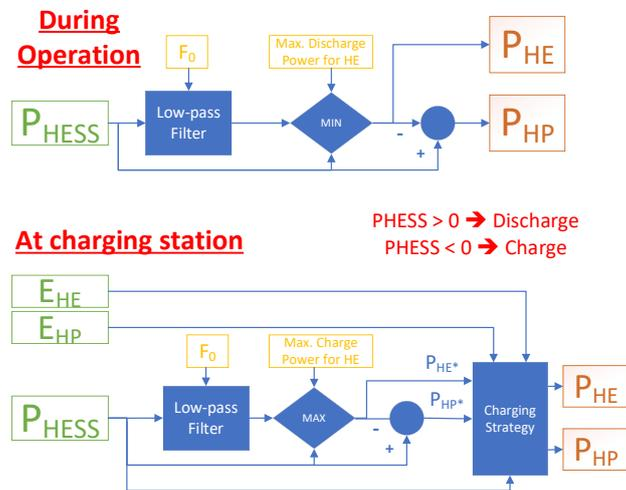
FIG. 6.4: POWER SPLIT STRATEGY BASED ON LOW PASS FILTERING FOR ZERO-EMISSION VESSELS. (TOP: STRATEGY DURING HESS DISCHARGING; BOTTOM: STRATEGY DURING HESS CHARGE OPERATION AT CHARGING STATION)
