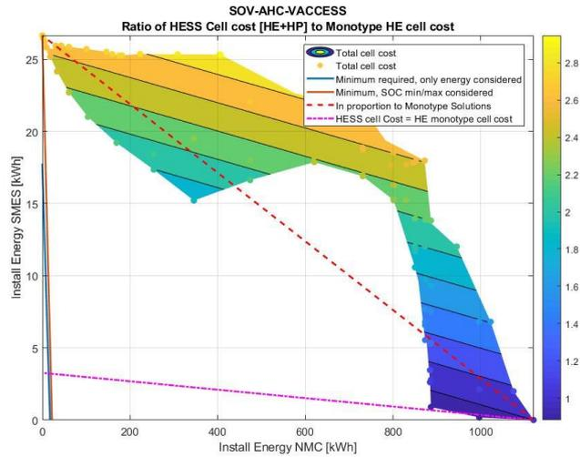
**FIG. 10.45: HESS SCREENING RESULTS FOR OSV-AHC CASE WITH NMC BATTERIES AND SMES. GENSET LFP = 0,01Hz. (NMC DESIGN LIFE = 10 YEARS)**
