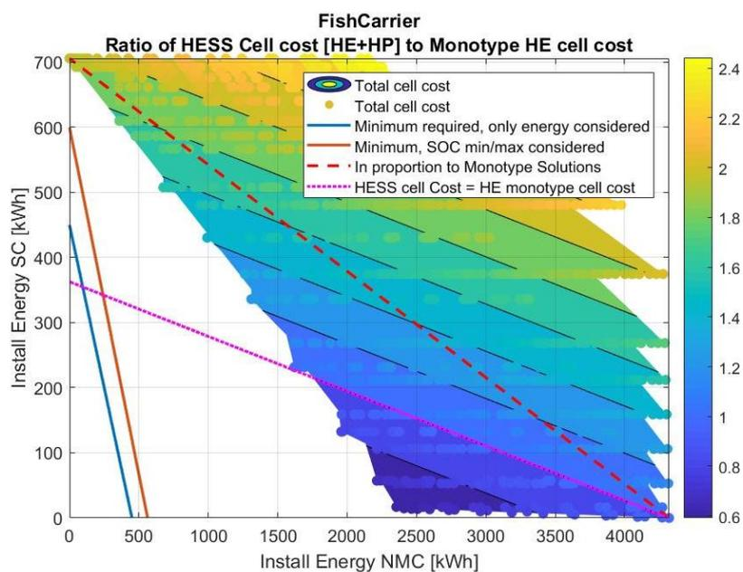
**FIG. 10.32: HESS SCREENING RESULTS FOR FISH CARRIER CASE WITH NMC BATTERIES AND SC. (SC & NMC DESIGN LIFE = 7.5 YEARS)**
