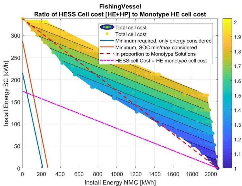
**FIG. 10.36: HESS SCREENING RESULTS FOR FISHING VESSEL CASE WITH NMC BATTERIES AND SC. (SC & NMC DESIGN LIFE = 7.5 YEARS)**
