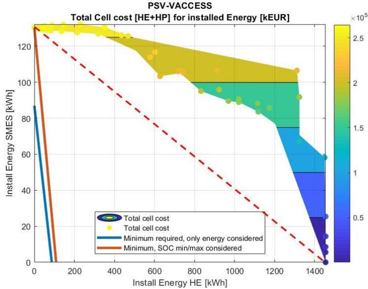
FIG. 10.11: HESS SCREENING RESULTS FOR PSV CASE WITH NMC BATTERIES AND SMES. (LFP = 0.005Hz)
