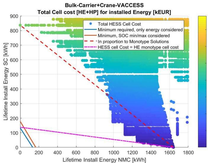
**FIG. 10.41: HESS SCREENING RESULTS FOR BULK CARRIER CRANE OPERATION CASE WITH NMC BATTERIES AND SC. LIFETIME INSTALLED CAPACITY FOR DIFFERENT DESIGN LIFE: NMC → 5-15 YEARS AND SC → 5- 7.5 YEARS.**
