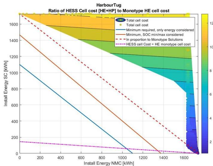
**FIG. 10.21: HESS SCREENING RESULTS FOR HARBOUR TUG CASE WITH NMC BATTERIES AND SC. (SC & NMC DESIGN LIFE = 7.5 YEARS)**
