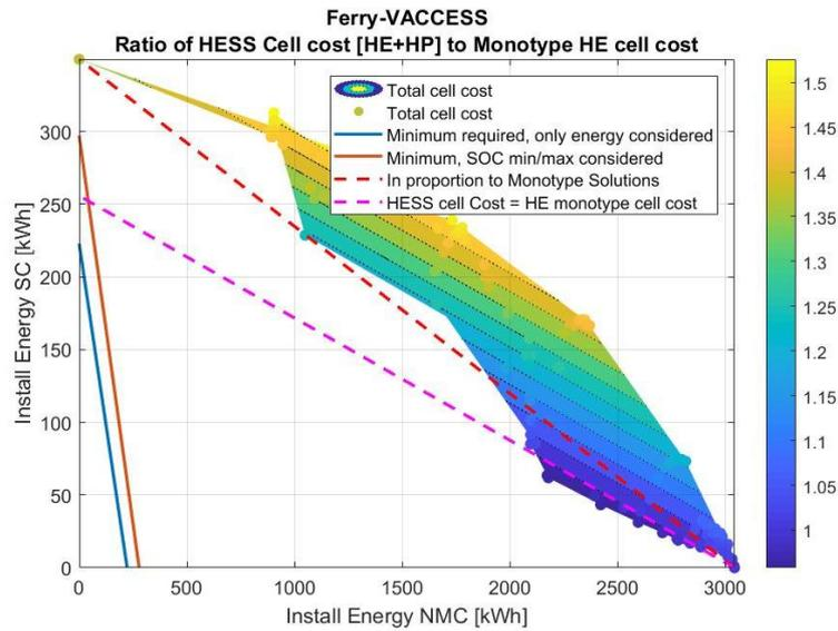
**FIGURE 10-5: HESS SCREENING RESULTS FOR FERRY CASE WITH NMC BATTERIES AND SUPERCAPACITORS. RESULTS FOR NMC AND SC DESIGN LIFE OF 7.5 YEARS.**
