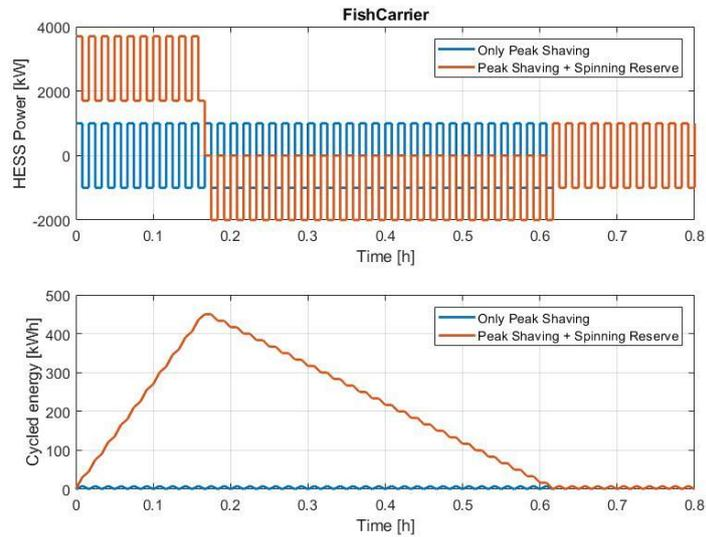
**FIG. 10.30: FISH CARRIER - FUNDAMENTAL CYCLES**
