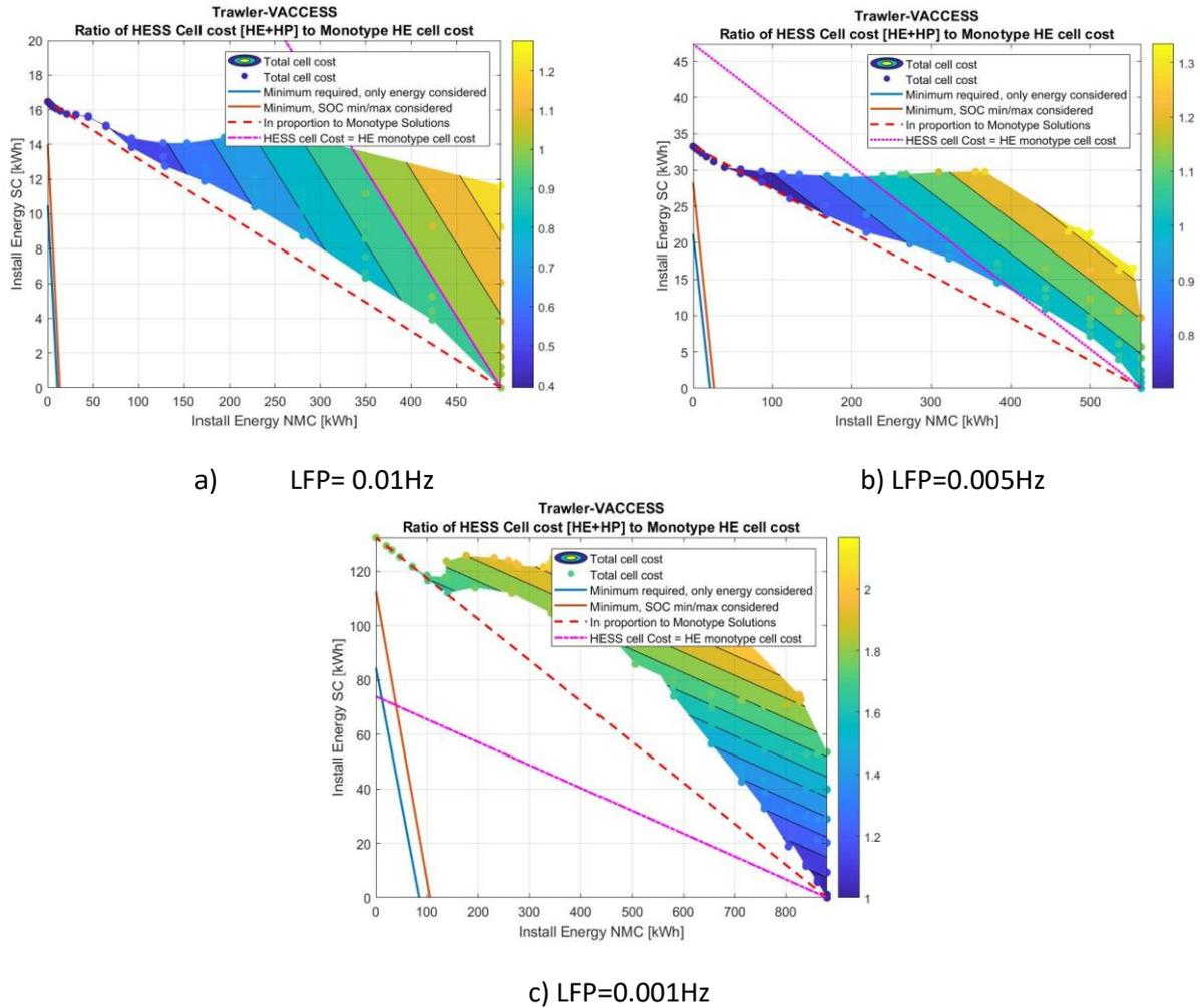
**FIG. 10.14: HESS SCREENING RESULTS FOR TRAWLER CASE WITH NMC BATTERIES AND SC.**
