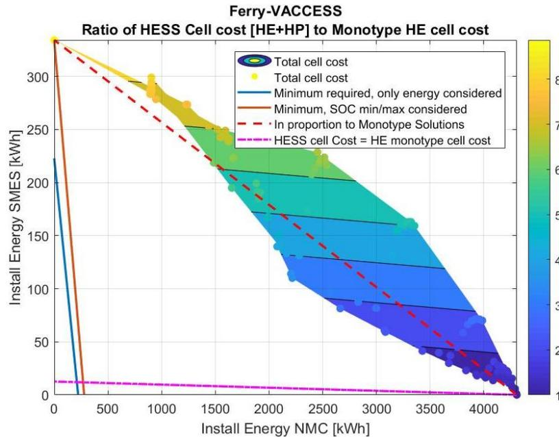
**FIG. 10.7: HESS SCREENING RESULTS FOR FERRY CASE WITH NMC BATTERIES AND SMES. RESULTS FOR NMC DESIGN LIFE OF 10 YEARS AND SMES DESIGN LIFE EQUAL TO SHIP LIFETIME (30 YEARS).**
