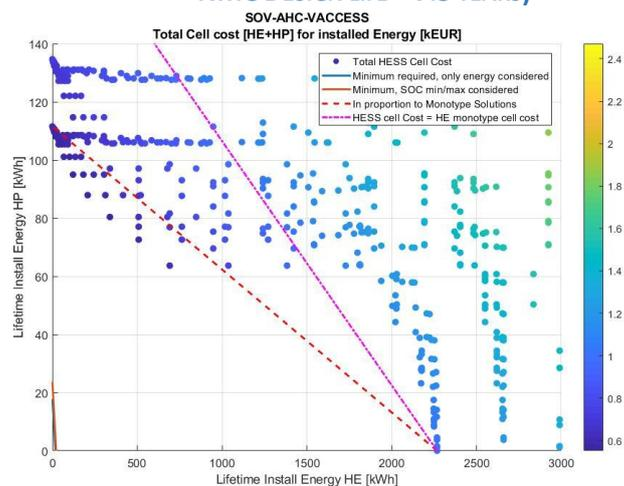
**FIG. 10.44: HESS SCREENING RESULTS FOR OSV-AHC CASE WITH NMC BATTERIES AND SC. LIFETIME INSTALLED CAPACITY FOR DIFFERENT DESIGN LIVES: NMC → 5-15 YEARS AND SC → 5- 7.5 YEARS.**
