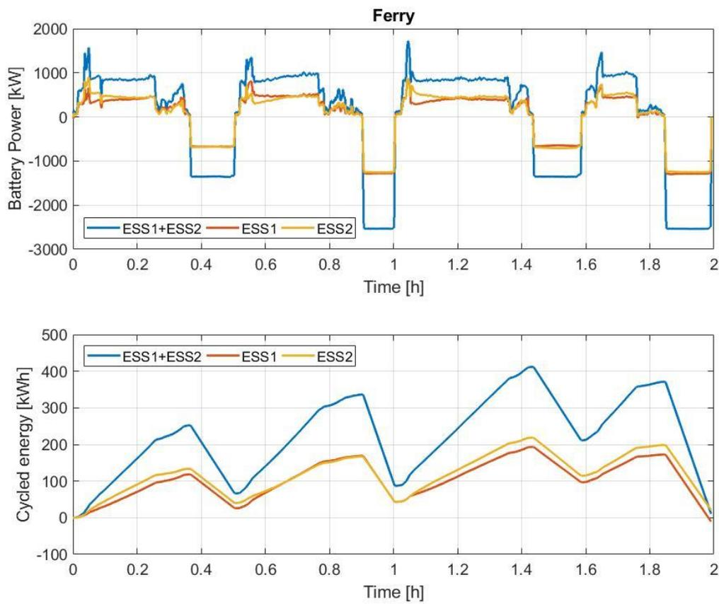
FIGURE 10-3: FERRY - FUNDAMENTAL CYCLE
