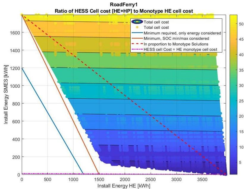
**FIG. 10.17: HESS SCREENING RESULTS FOR RO-RO FERRY 1 CASE WITH NMC BATTERIES AND SMES. NMC DESIGN LIFE = 10 YEARS**
