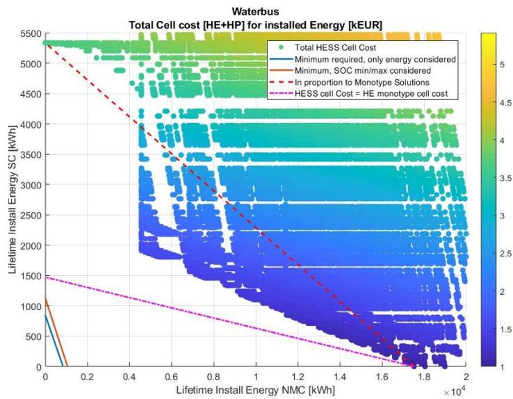
**FIG. 10.27: HESS SCREENING RESULTS FOR WATER BUS CASE WITH NMC BATTERIES AND SC. LIFETIME INSTALLED CAPACITY FOR DIFFERENT DESIGN LIFE: NMC → 5-15 YEARS AND SC → 5- 7.5 YEARS.**
