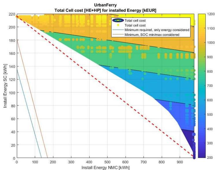
**FIGURE 10.24: HESS SCREENING RESULTS FOR URBAN FERRY CASE WITH NMC BATTERIES AND SC. (SC & NMC DESIGN LIFE = 7.5 YEARS)**
