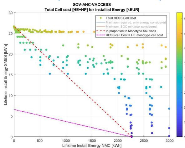
**FIG. 10.46: HESS SCREENING RESULTS FOR OSV-AHC CASE WITH NMC BATTERIES AND SMES. LIFETIME INSTALLED CAPACITY FOR DIFFERENT DESIGN LIFES: NMC → 5-15 YEARS AND SMES = 30 YEARS (SHIP LIFETIME).**
