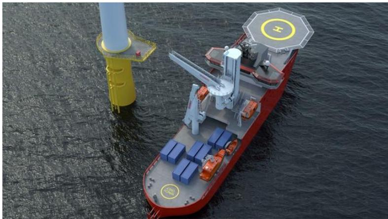
**FIG.5.3: GANGWAY AT WINDMILL– CREDIT VARD DESIGN**
