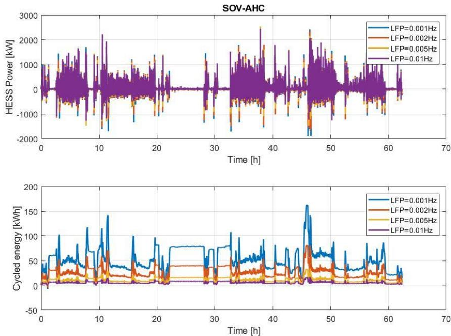
**FIG. 10.42: POSSIBLE OSV-AHC HESS POWER PROFILE FOR DIFFERENT LOW PASS FILTER CUT-OFF FREQUENCIES**
