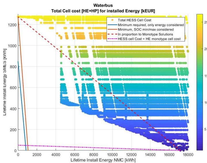
**FIG. 10.29: HESS SCREENING RESULTS FOR WATER BUS CASE WITH NMC BATTERIES AND SMES. LIFETIME INSTALLED CAPACITY FOR DIFFERENT DESIGN LIFE: NMC → 5-15 YEARS AND SMES → SHIP LIFETIME (30 YEARS).**
