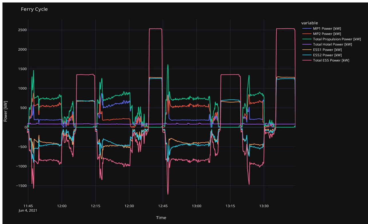
FIGURE A-4 ELECTRIC FERRY LOG DATA PROVIDED BY VARD ELECTRIC
